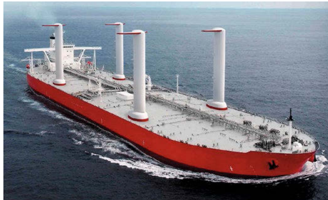
The partners plan to develop Suction Wings over a range of sizes for different vessel types Source: Bureau Veritas
