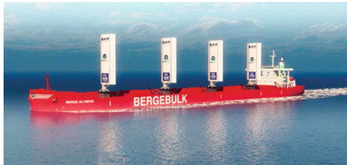
The Newcastlemax bulk carrier, Berge Olympus , will be equipped with four WindWings Source: Yara Marine Technologies
