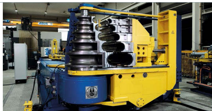
Heavy Duty tube and pipe bending machine CNC 220 HD with multi-stack bending tool
