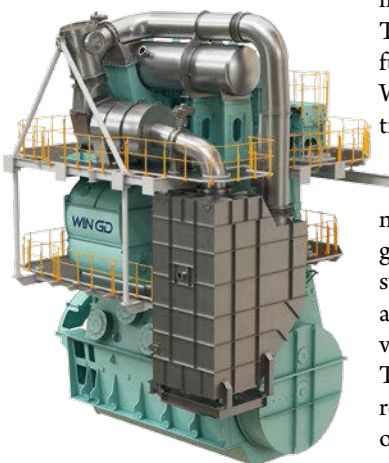
Intelligent Control by Exhaust Recycling (iCER) is the first technology launched on the X-DF2.0 platform
