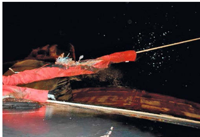
Broken ropes with the SBA still intact. This feature prevented highly dangerous snap back.
